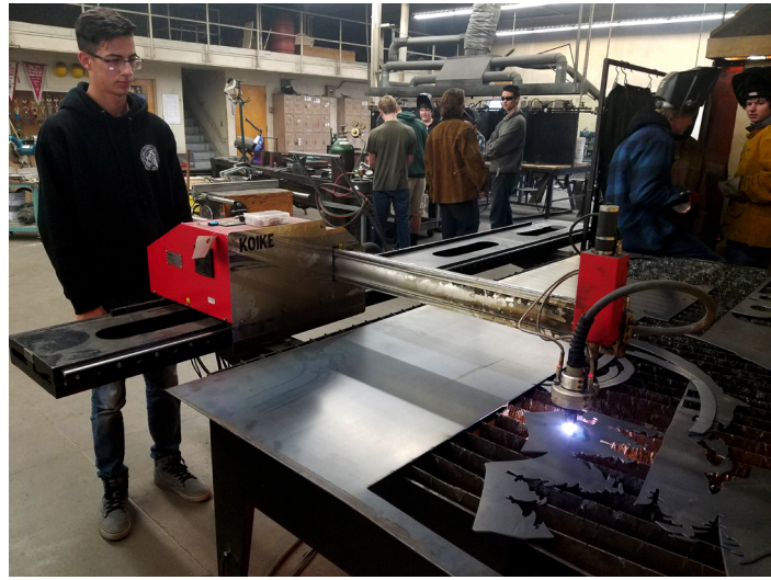
Matt Pritchard's Ag Mechanics plasma cutter doing its job.
